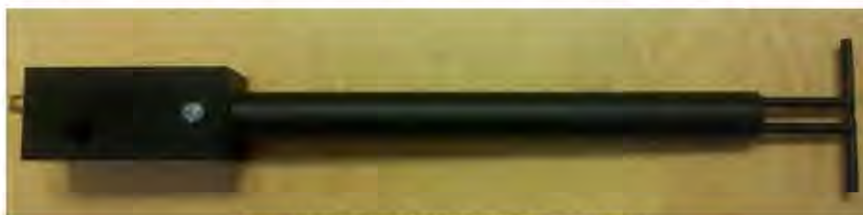
Figure 1 – MVG COMOSAR Validation Dipole
