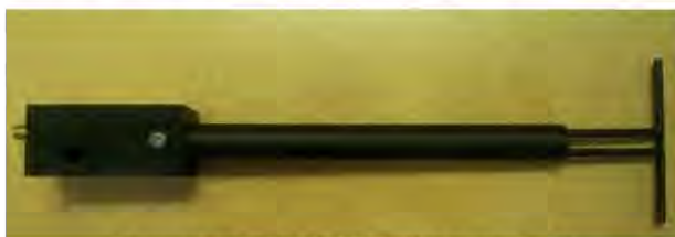
Figure 1 – MVG COMOSAR Validation Dipole
