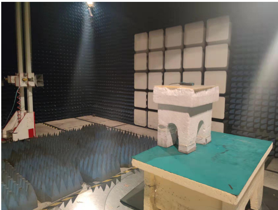
Spurious Emission Test Setup (Above 1GHz)
