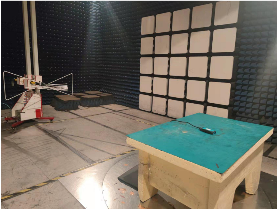
Spurious Emission Test Setup (Below 1GHz)
