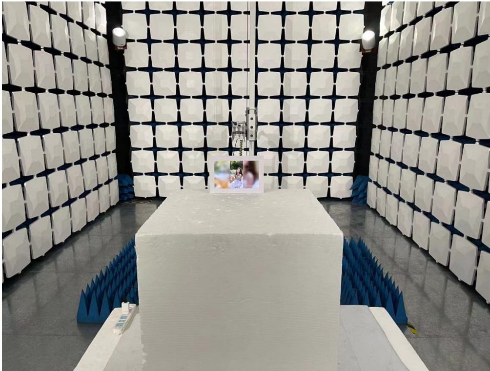
Above 1GHz for radiated emission test setup
