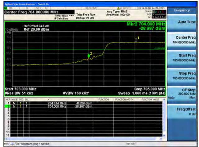
Band17 / 5MHz / High CH / QPSK / FULL RB
