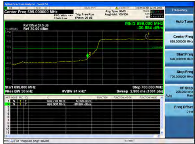
Band12 / 1.4MHz / High CH / QPSK / FULL RB
