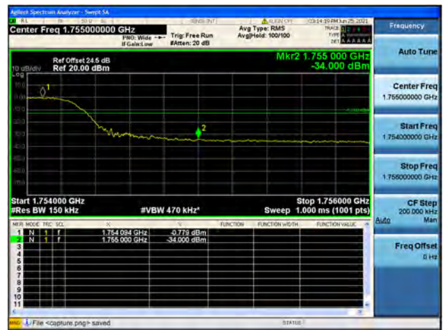
Band4 / 15MHz / High CH / QPSK / FULL RB
