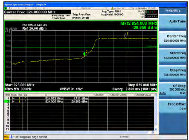
Band5 / 1.4MHz / High CH / QPSK / FULL RB
