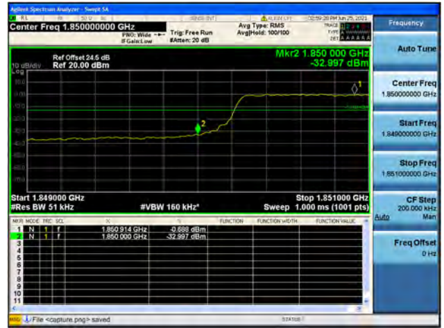
Band2 / 5MHz / High CH / QPSK / FULL RB
