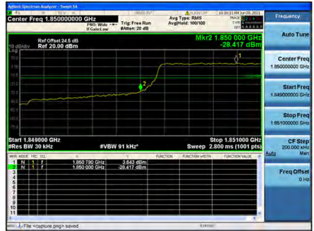
Band25 / 1.4MHz / High CH / QPSK / FULL RB
