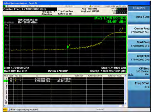
Band4 / 15MHz / High CH / QPSK / FULL RB
