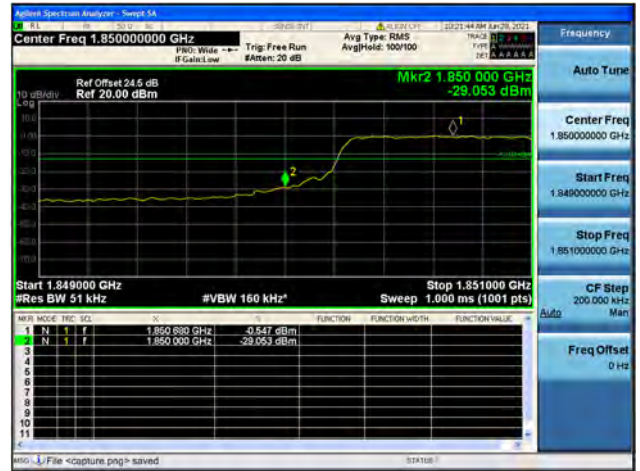
Band25 / 5MHz / High CH / QPSK / FULL RB
