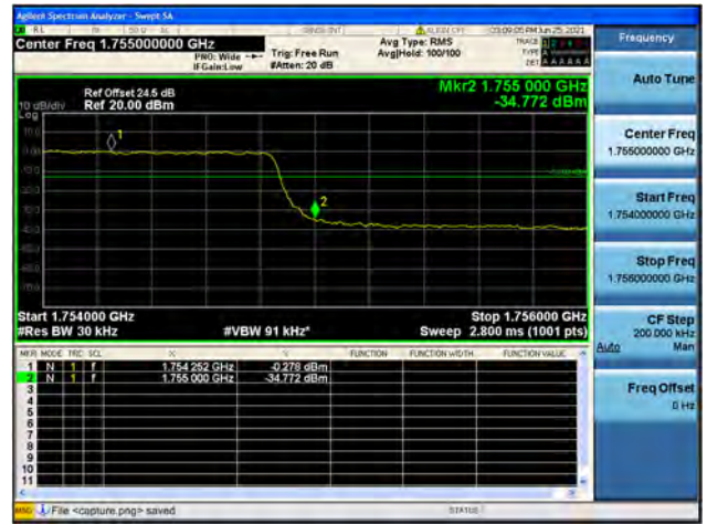
Band4 / 3MHz / High CH / QPSK / FULL RB
