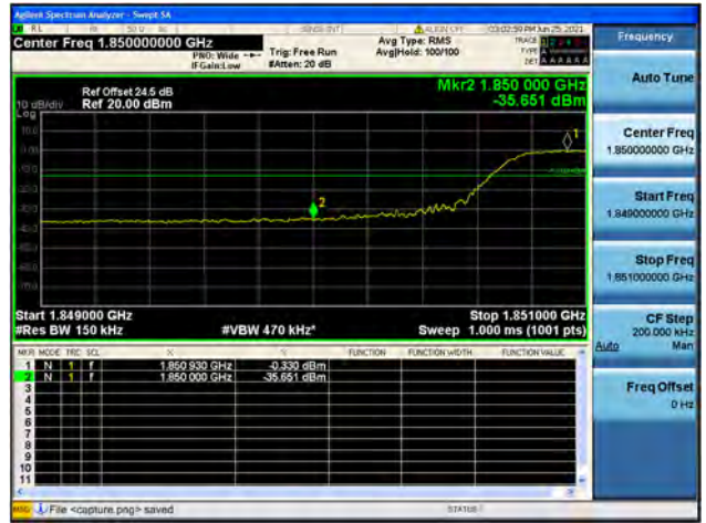
Band2 / 15MHz / High CH / QPSK / FULL RB
