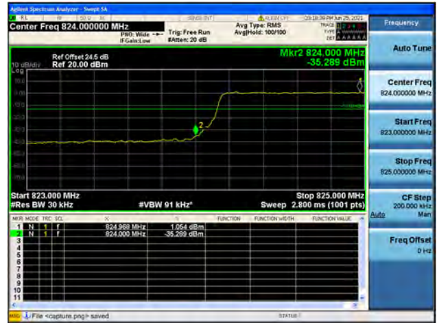
Band5 / 3MHz / High CH / QPSK / FULL RB
