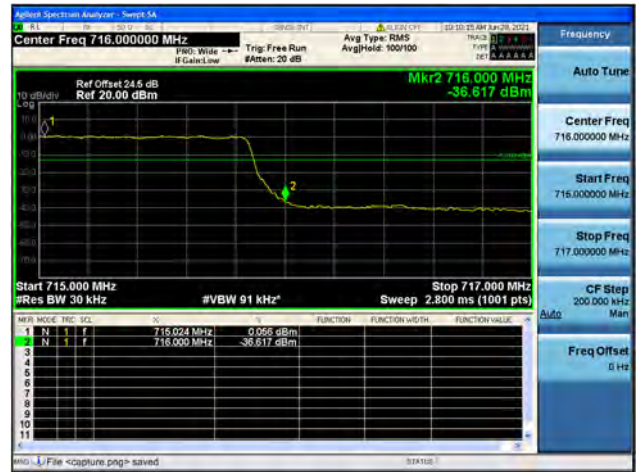
Band12 / 3MHz / High CH / QPSK / FULL RB
