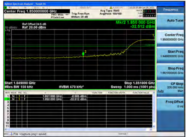
Band25 / 15MHz / High CH / QPSK / FULL RB
