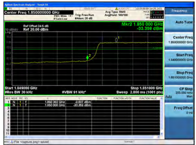
Band25 / 3MHz / High CH / QPSK / FULL RB
