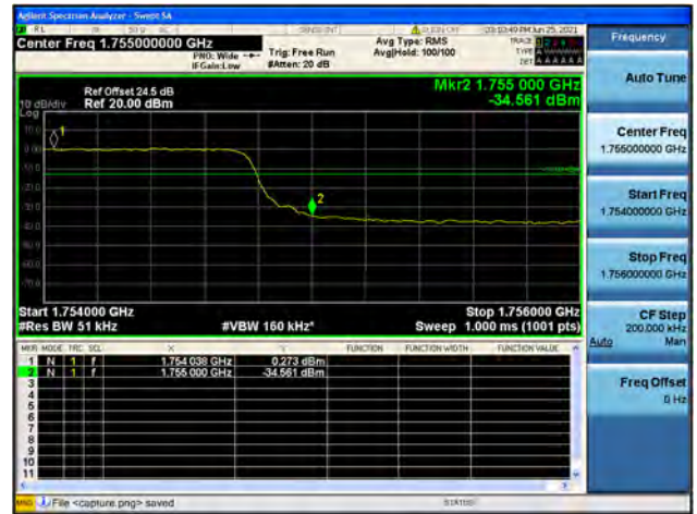
Band4 / 5MHz / High CH / QPSK / FULL RB
