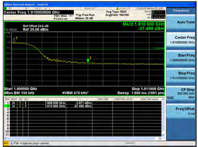
Band2 / 15MHz / High CH / QPSK / FULL RB
