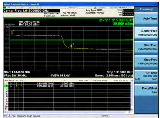
Band25 / 3MHz / High CH / QPSK / FULL RB
