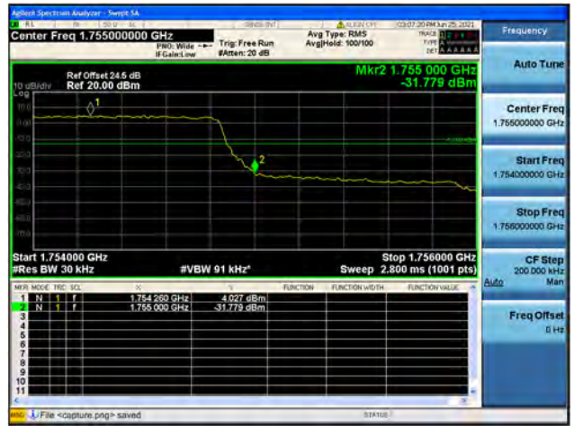
Band4 / 1.4MHz / High CH / QPSK / FULL RB
