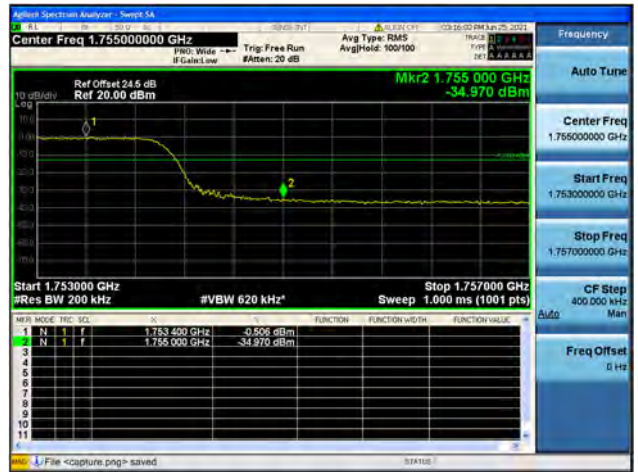
Band4 / 20MHz / High CH / QPSK / FULL RB
