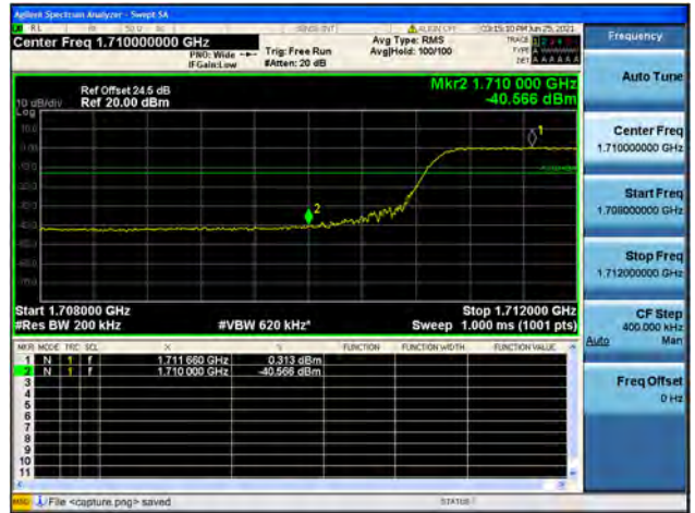
Band4 / 20MHz / High CH / QPSK / FULL RB
