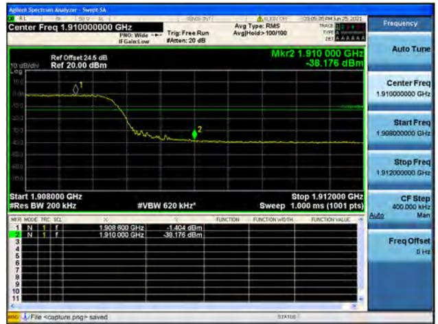
Band2 / 20MHz / High CH / QPSK / FULL RB
