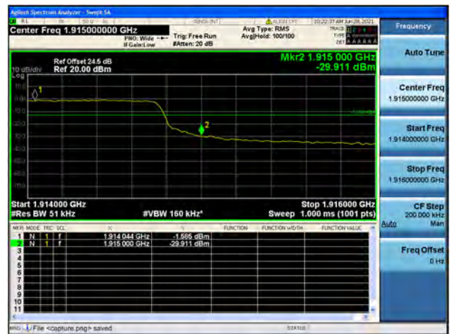
Band25 / 5MHz / High CH / QPSK / FULL RB
