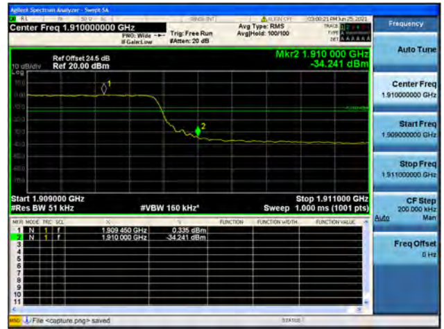
Band2 / 5MHz / High CH / QPSK / FULL RB
