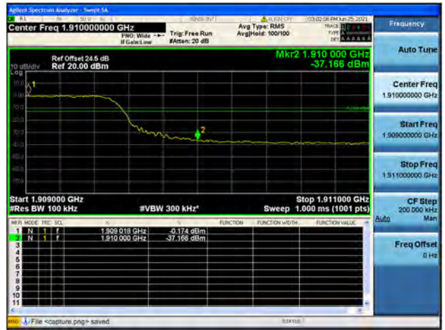
Band2 / 10MHz / High CH / QPSK / FULL RB
