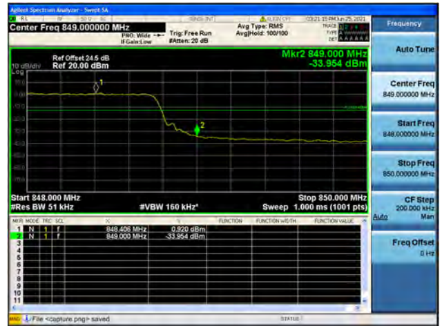
Band5 / 5MHz / High CH / QPSK / FULL RB
