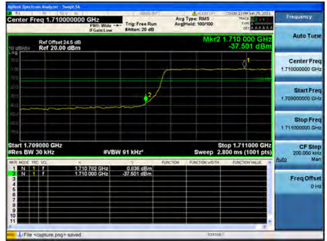
Band4 / 3MHz / High CH / QPSK / FULL RB
