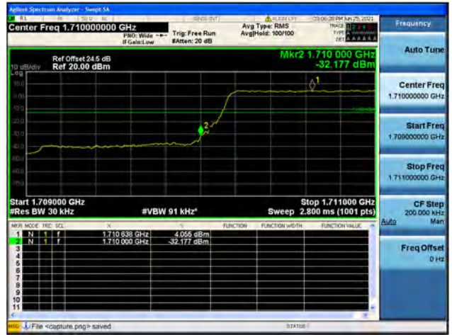
Band4 / 1.4MHz / High CH / QPSK / FULL RB
