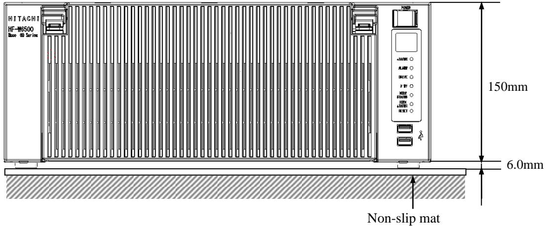
Figure 1-6 Exterior View (Horizontal Installation on the Desktop)
