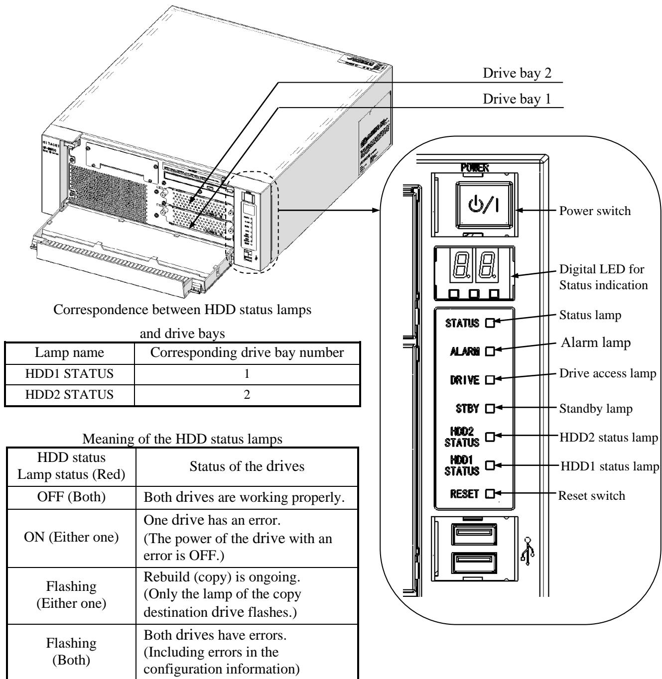
Figure 10-1 HDD status lamp
