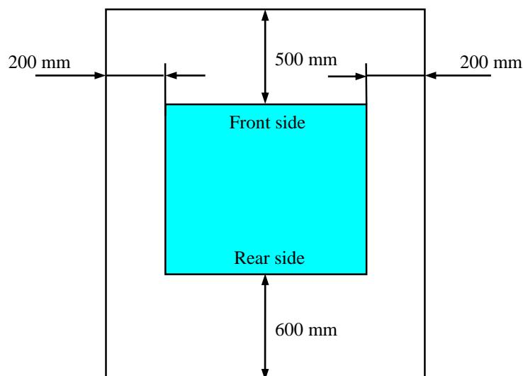
Figure 1-4 Operation and Service Clearance (Top View)
