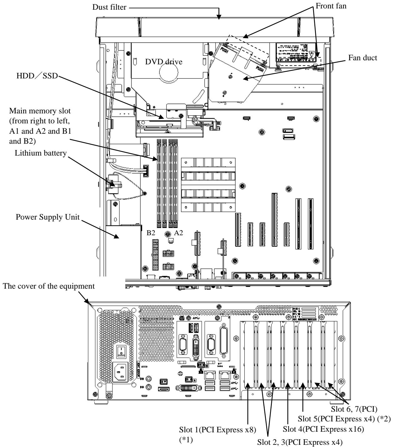
(\*1) A PCI Express x8 connector is used but the internal connection is equivalent to PCI Express x4.
