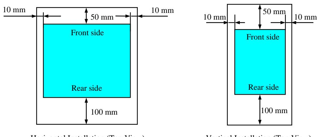
Figure 1-5 Installation Clearance
