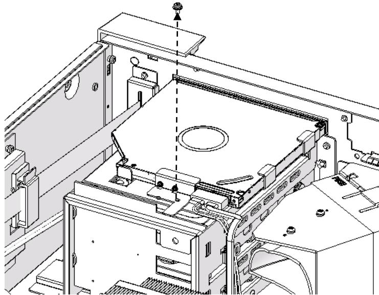
Figure 6-9 Removing the screw fixing the DVD drive
