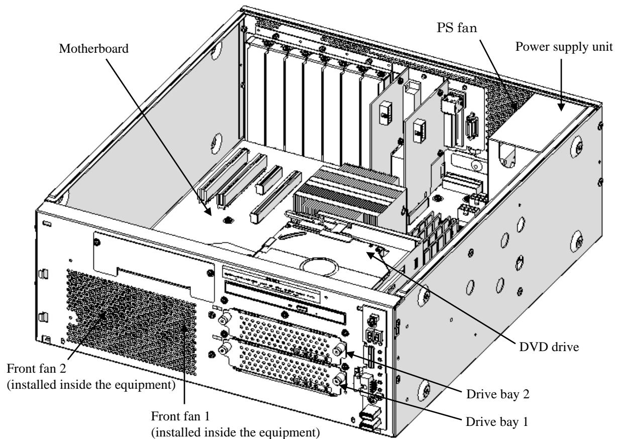
Figure 1-3 Physical Configuration Inside Equipment
