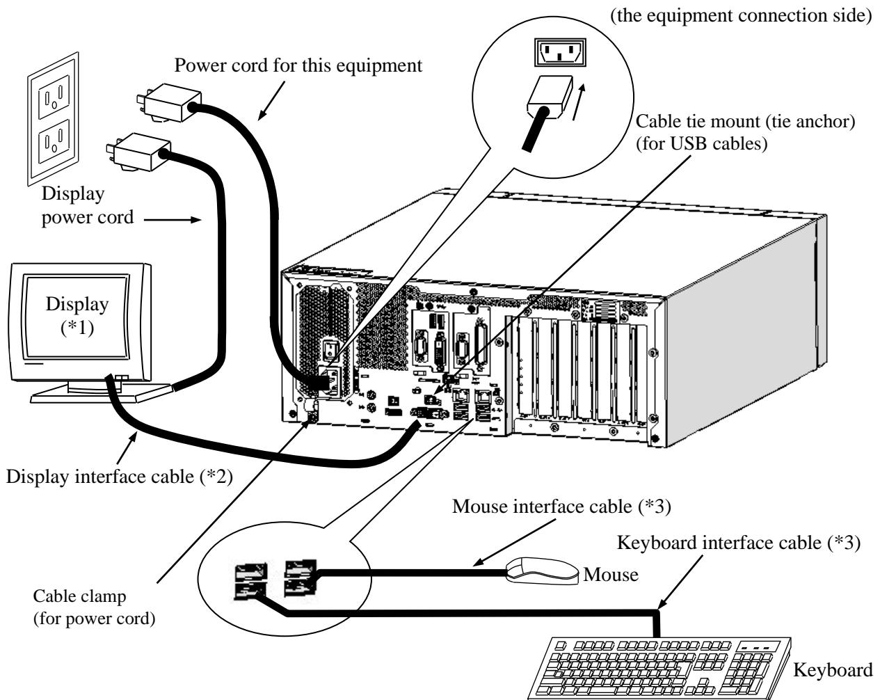
Figure 1-9 Hardware Connection
