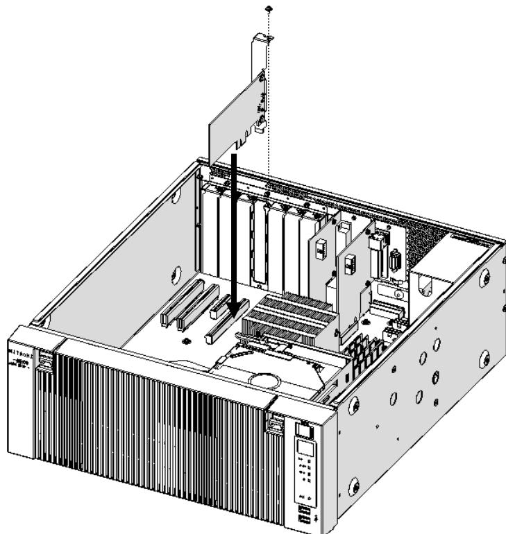
Figure 6-3 Installing an extension board
