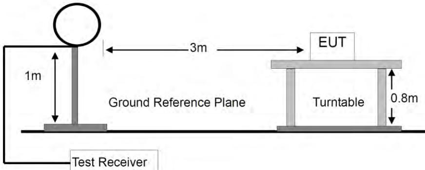
For Radiated Emission 30-1000MHz
