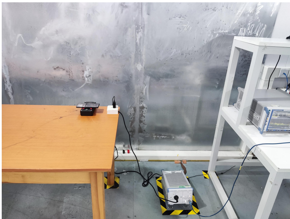
Conducted Emission-AC adapter charge mode
