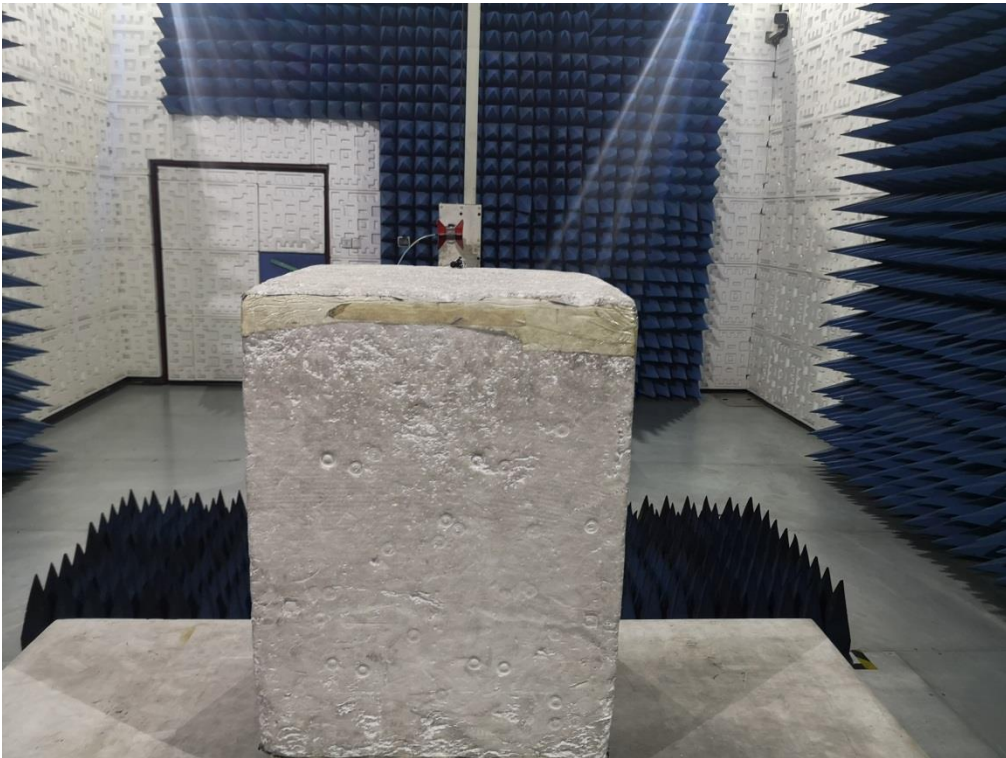
RADIATED EMISSION TEST SETUP ABOVE 1GHz
