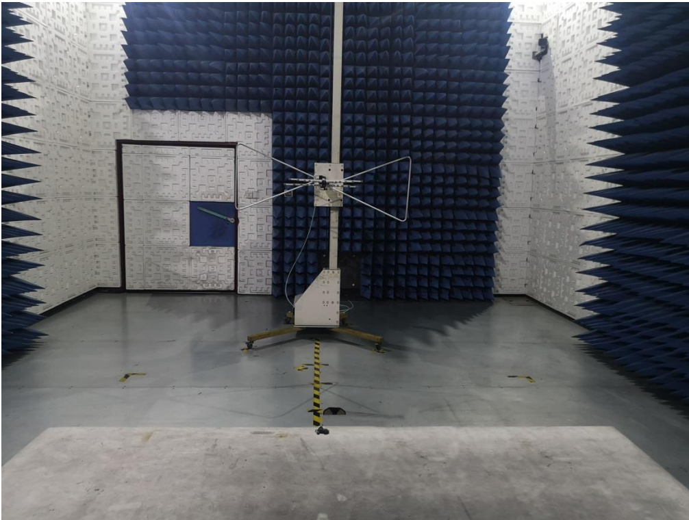
RADIATED EMISSION TEST SETUP ABOVE 1GHz
