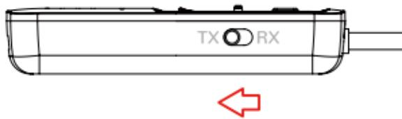
RX/TX mode switch push to TX side
