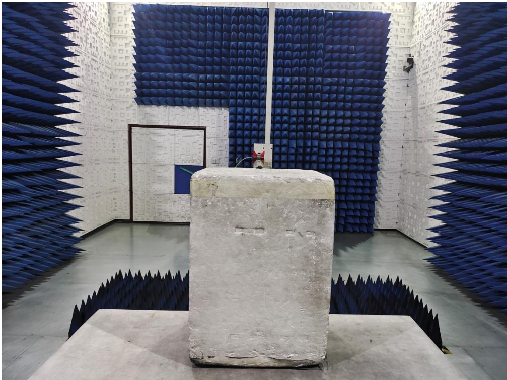
RADIATED EMISSION TEST SETUP ABOVE 1GHz
