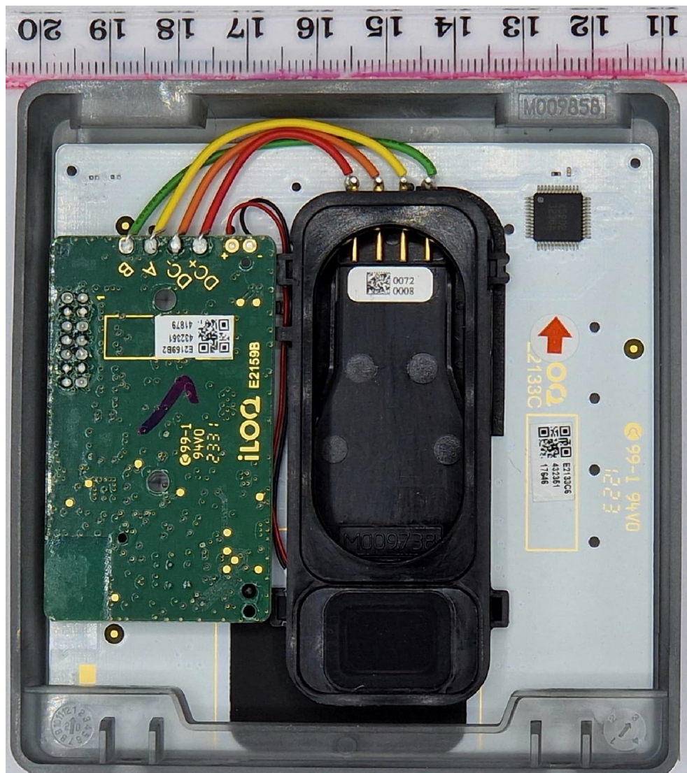
Figure 1: Internal view without potting.
