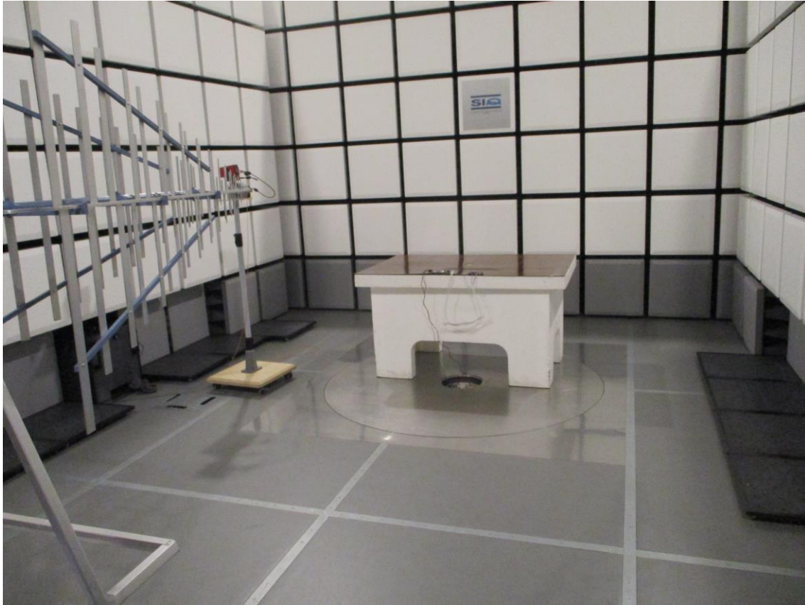
Figure 3: Spurious emission 30 MHz-1000 MHz
