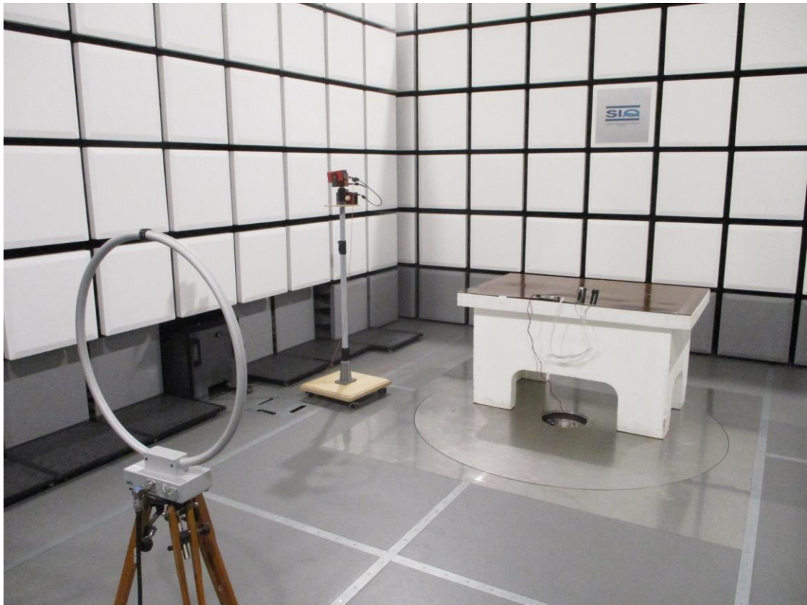
Figure 1: Spurious emission 9 kHz - 30 MHz
