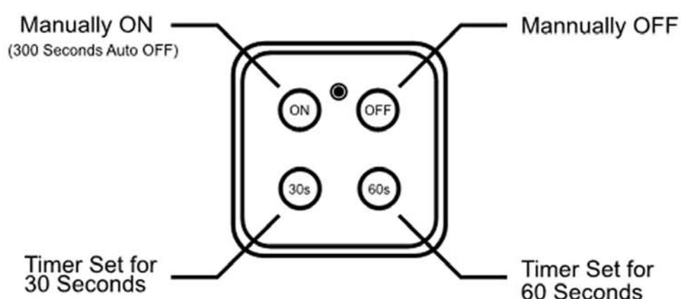
How to disable the air switch and use the wireless socket? Most of the waste disposers are shipped with the switch in the "off" position from the disposer manufacturer. So you need to disable the air switch before using the wireless socket.
