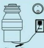
Plug disposer cord into power module.
