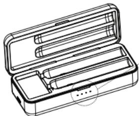
\*When there is no transmitter/receiver charging, as long as opening the charging case, the power indicator LED will be lightened to show the current electric quantity for 5 seconds
