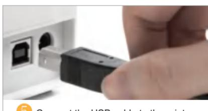
5 Connect the USB cable to the printer
