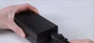
2 Attach the power cord to the adapter
