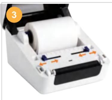
Put the roll label in or insert the fan-fold label from outside, adjust the paper guide to fit the width of paper.
