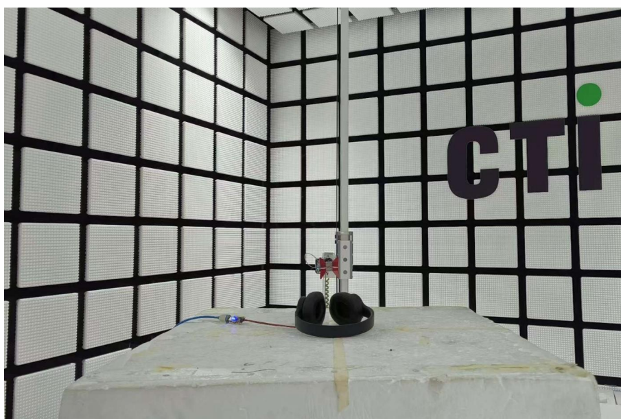
Radiated spurious emission Test Setup-2(Above 1GHz)
