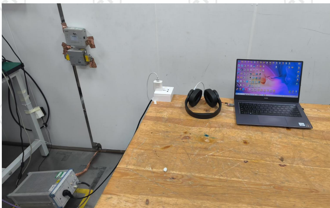
AC Power Line Conducted Emissions Test Setup
