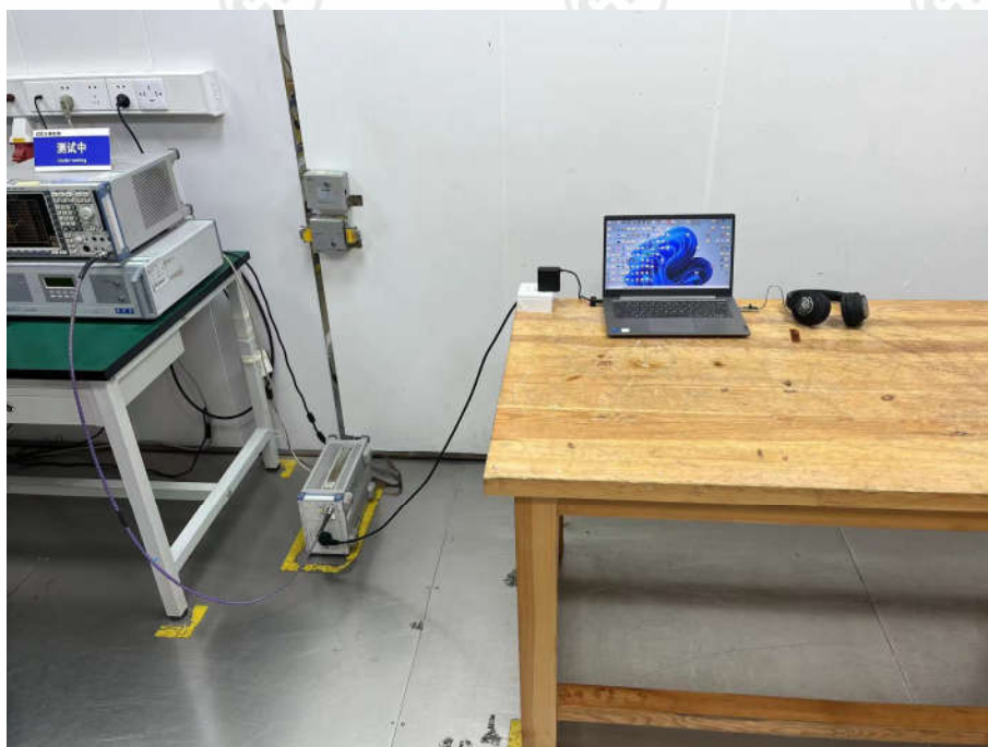
Conducted Emissions Test Setup
