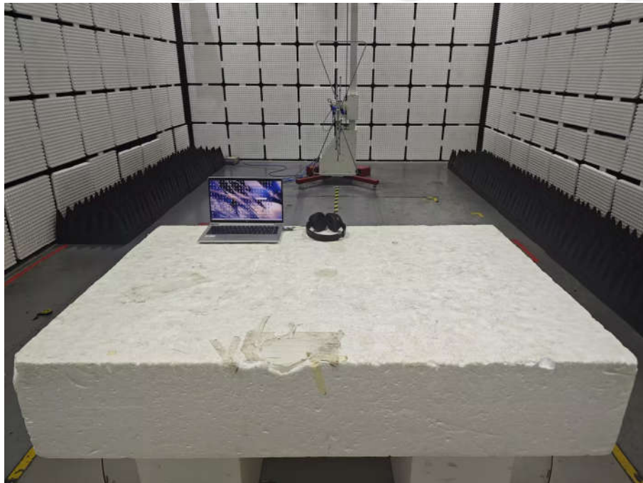
Radiated spurious emission Test Setup-1(Below 1GHz)
