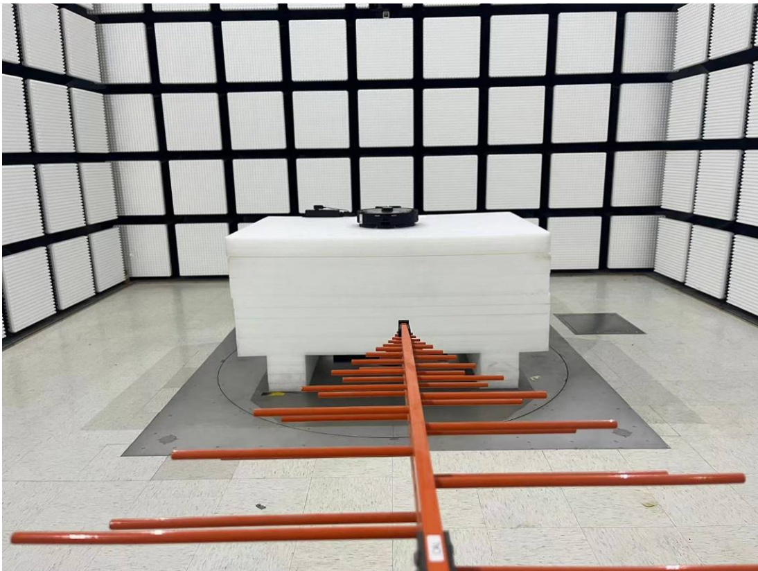
Radiated Emission Below 1GHz View - Test with iHRVS2-3BLKS Charging Station
