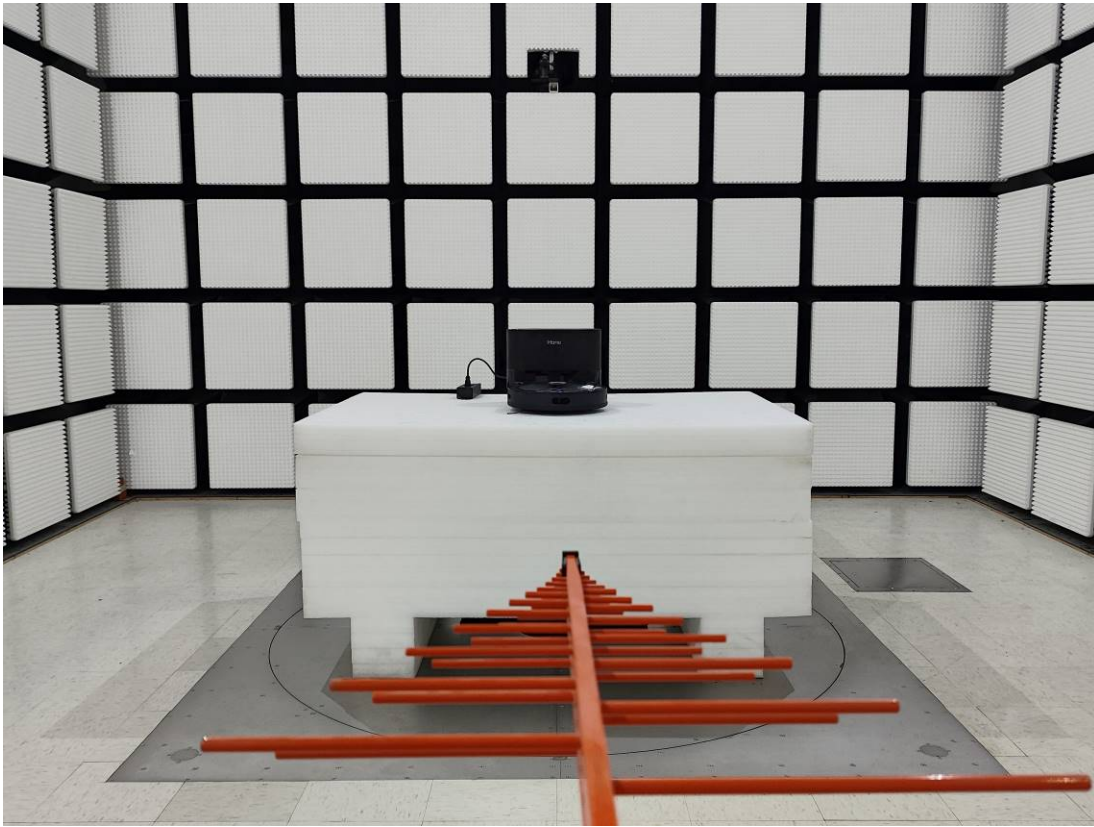
Radiated Emission Below 1GHz View - Test with iHRVS2-3BLKS Charging Station
