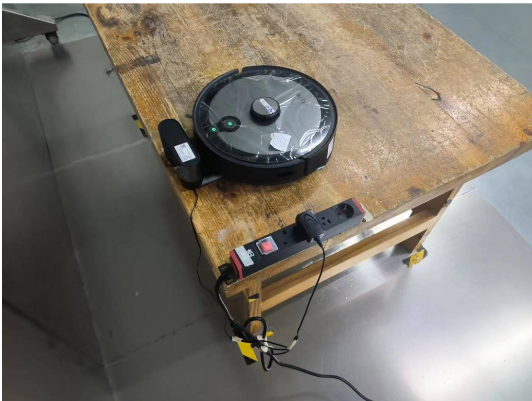
Conducted Emissions Side View- Test with iHRVS2-3BLKS Charging Station
