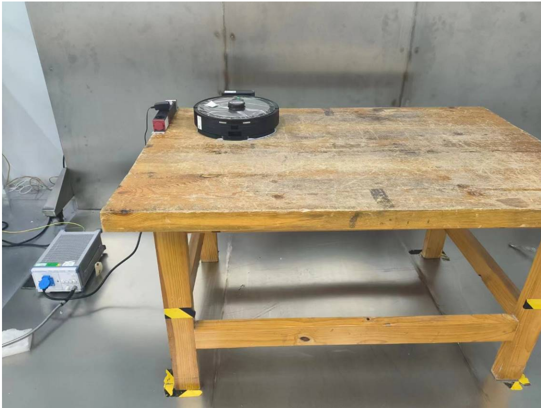
Conducted Emissions Side View- Test with iHRVS2-3BLKS Charging Station
