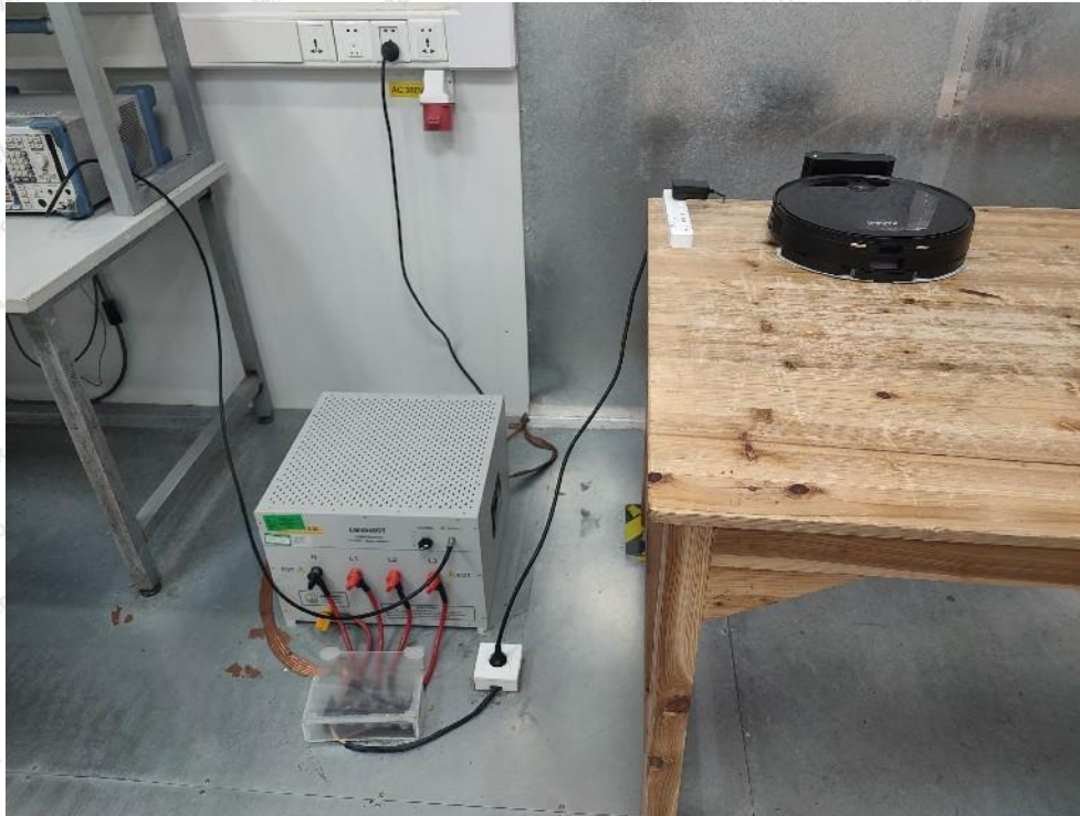
Photo of Power Line Conducted Emission Test
