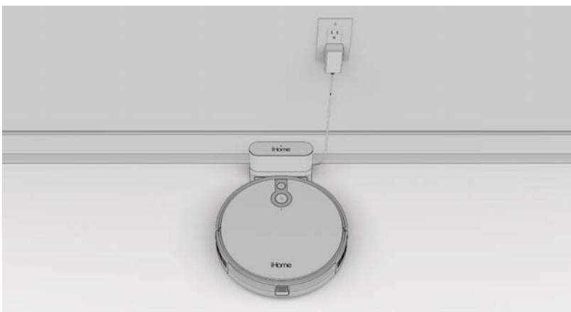
**NOTE:** Allow your Vacuum to fully charge (up to 5 hours) before first use. The indicators on your robot will turn solid green when fully charged.
