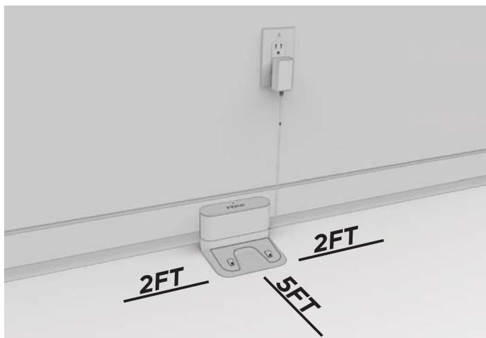
Place the charging dock against the wall and make sure the place is an open & uncluttered area. Leaving at least 5 feet in front of the charging dock and 2 feet on both sides of the charging dock.
