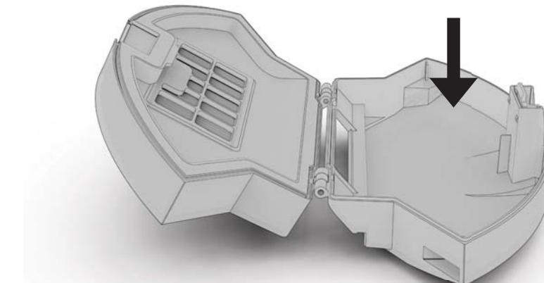
③ Remove the sponge filter and HEPA filter. Tap the HEPA filter to dislodge dust. Rinse the sponge filter and wipe down the filter housing with a dry cloth. Allow sponge filter to dry completely before reassembly.
