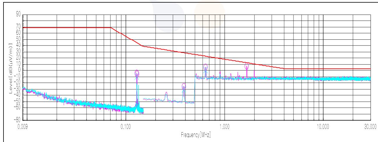
**IC Radiated Emissions Fundamental & 30 MHz to 1 000 MHz**
