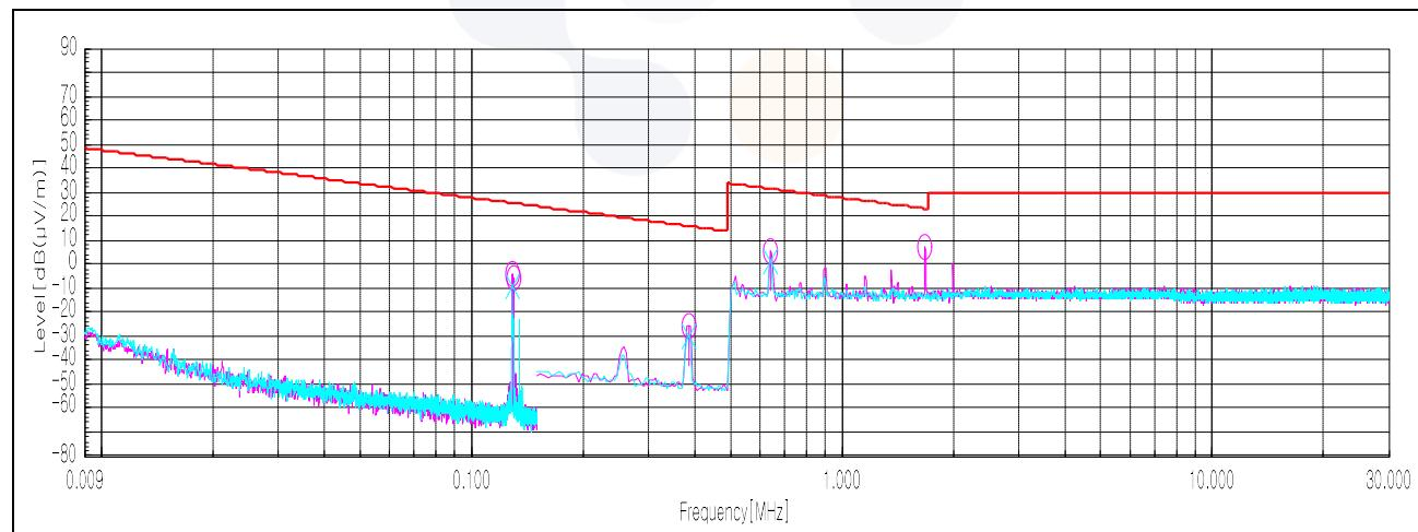
**IC Radiated Emissions Fundamental & 9 kHz to 30 MHz**
