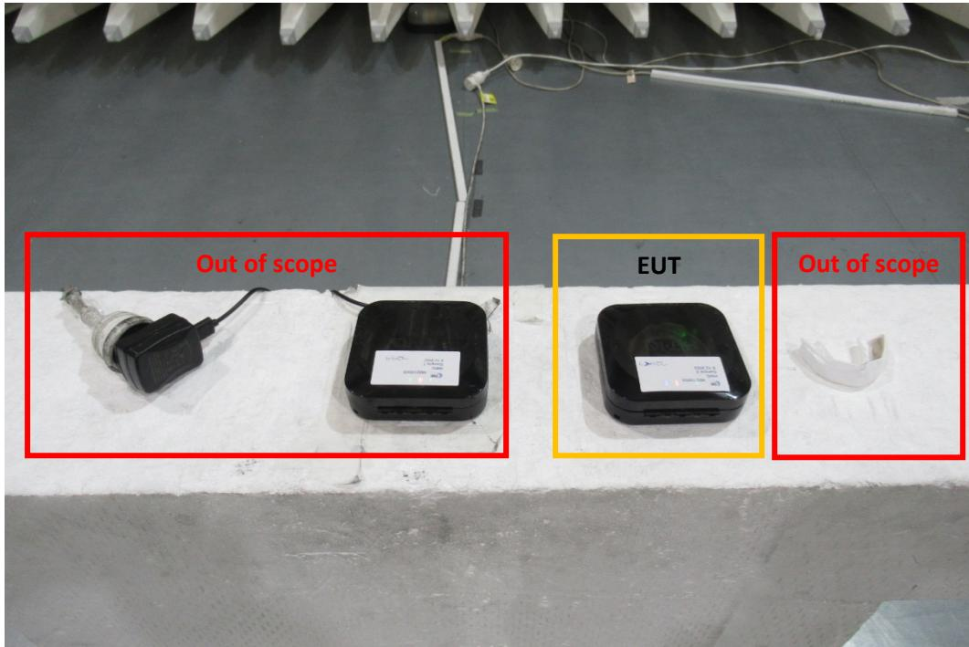
Radiated emission above 30MHz was conducted with other test samples to cover other EMC standards. This report only covers the WPT function of the EUT.
