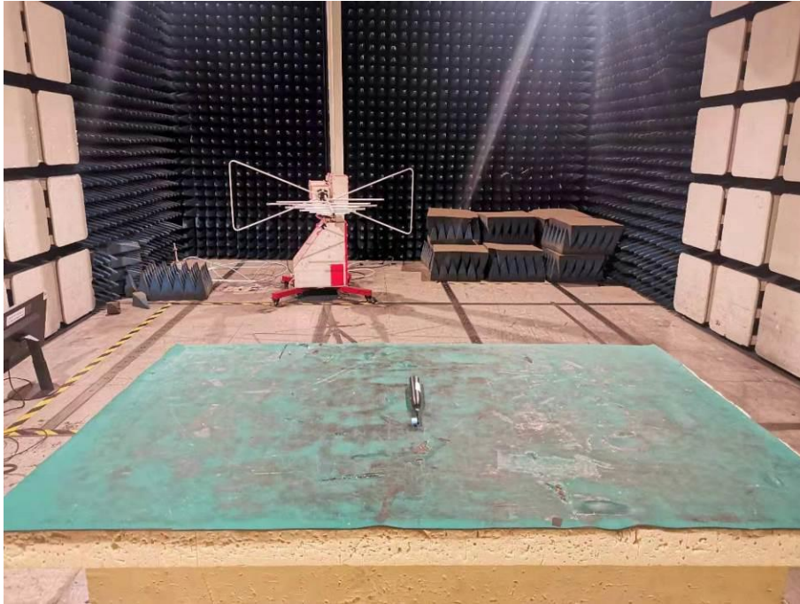
Spurious Emission Test Setup (Below 1GHz)
