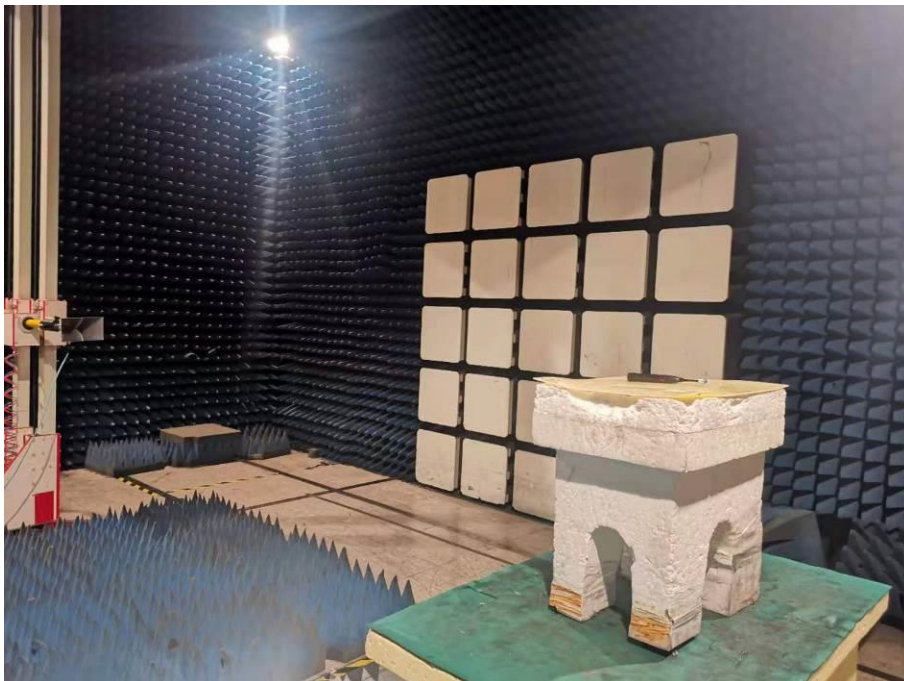
Spurious Emission Test Setup (Above 1GHz)
