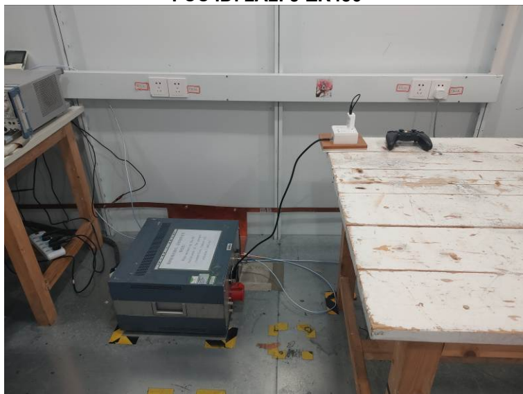
Test Setup Photo for Power Line Conducted Emissions
