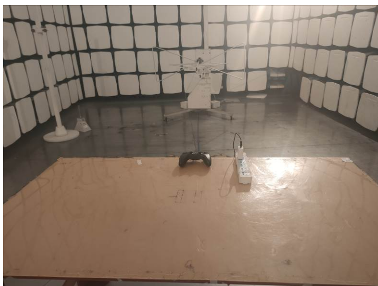
Test Setup Photo for Radiated Emissions (Below 1GHz)
