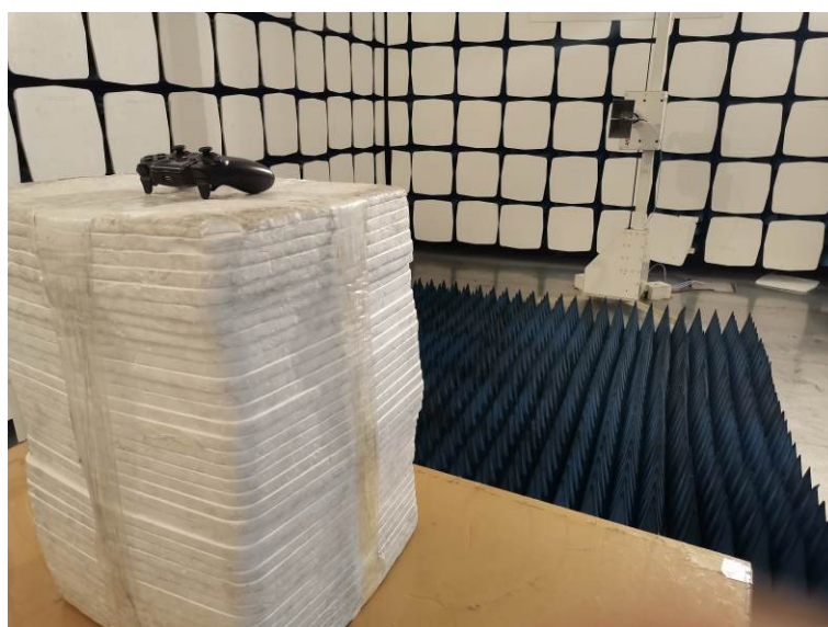
Test Setup Photo for Radiated Emissions (Above 1GHz)
