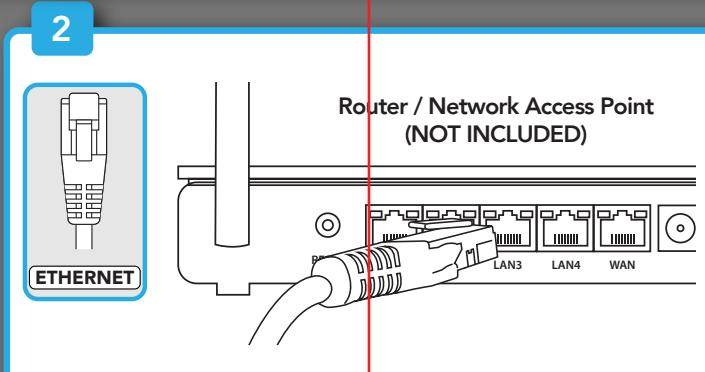
Plug the other end of the 6 ft. Ethernet cable into a port on the back of your router / network access point.
