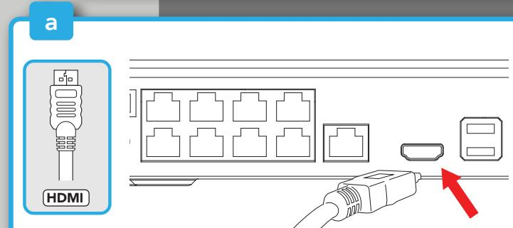
Plug one end of the included HDMI cable into the HDMI port on the back of the NVR. Plug the other end of the cable into your TV or Monitor.
