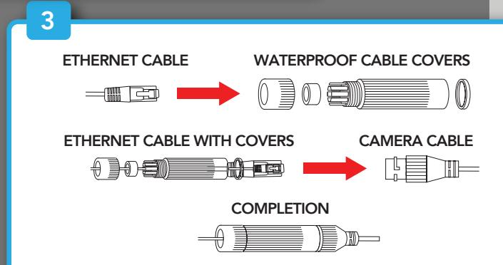
Insert one end of the wired IP camera's 60 ft. Ethernet cable into the cable covers. Connect the covered end of the Ethernet cable to the camera's power cable.
