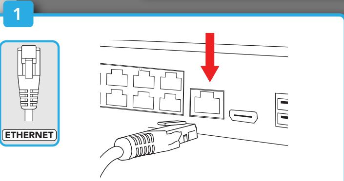
Plug one end of the included 6 ft. Ethernet cable into the LAN port on the back of the NVR.
