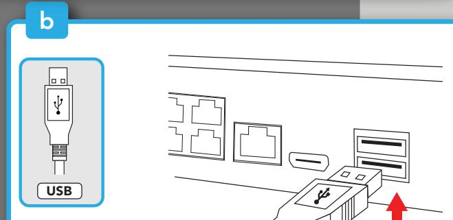
Plug the USB mouse into the USB port on the back of the NVR.
