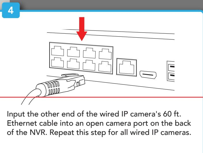
Input the other end of the wired IP camera's 60 ft. Ethernet cable into an open camera port on the back of the NVR. Repeat this step for all wired IP cameras.
