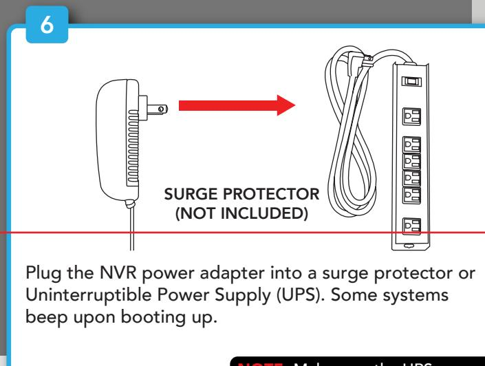
Plug the NVR power adapter into a surge protector or Uninterruptible Power Supply (UPS). Some systems beep upon booting up.
