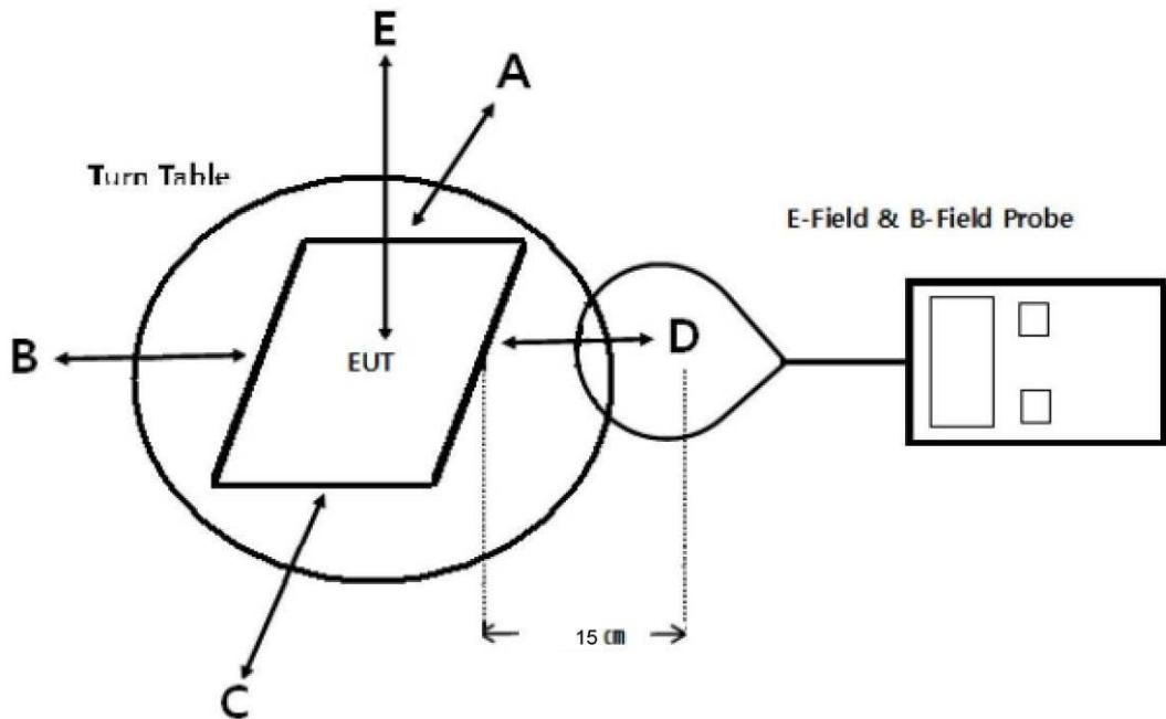
Note: Measurements should be made from all sides and the top of the primary/client pair, with the 15cm measured from the center of the probe(s) to the edge of the device.
