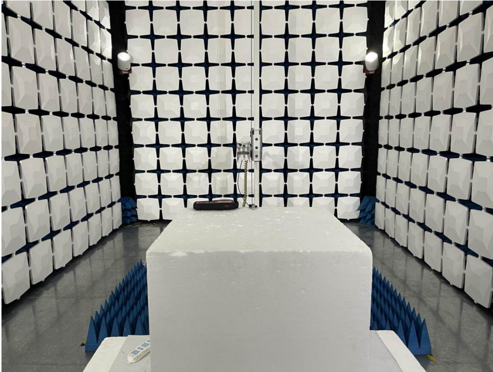
Above 1GHz for radiated emission test setup
