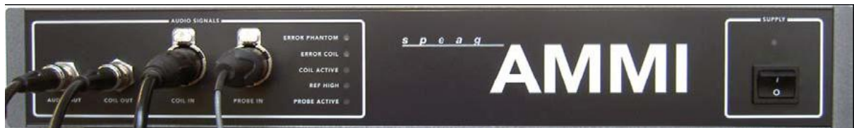
Figure 5.3 AMMI front panel
