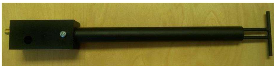
Figure 1 – MVG COMOSAR Validation Dipole
