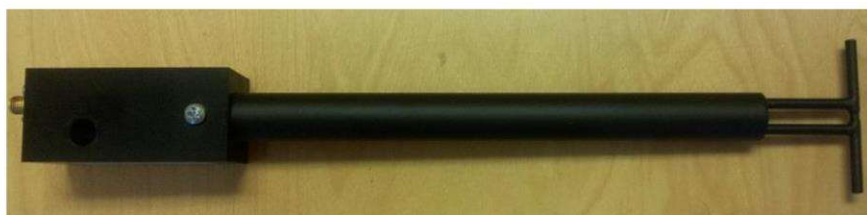
Figure 1 – MVG COMOSAR Validation Dipole
