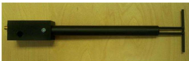
Figure 1 – MVG COMOSAR Validation Dipole
