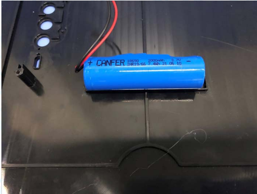
Photo 9 Appearance of Battery
