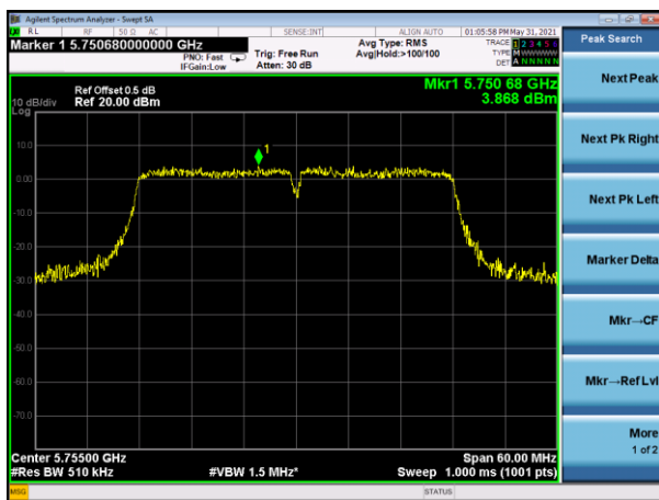
(802.11n40) PSD plot on channel 159
