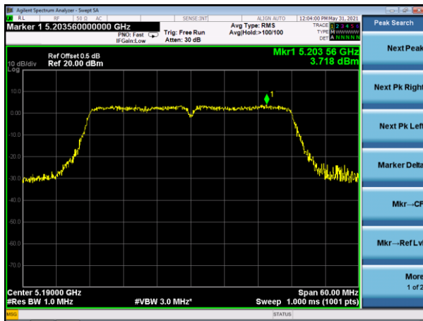
(802.11n40) PSD plot on channel 46
