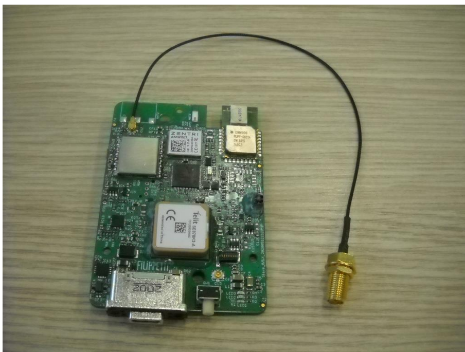
Figure 9.1-3: EUT modified with antenna connector for conducted test
