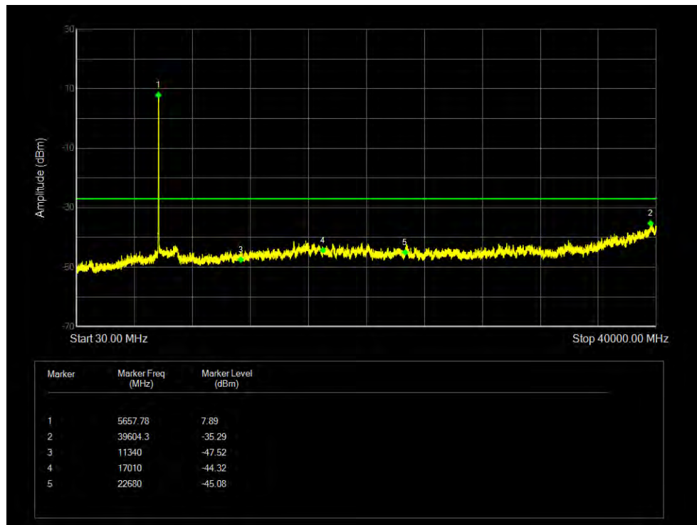
Tx. Spurious NVNT 802.11ac80 5530MHz Sum Emission
