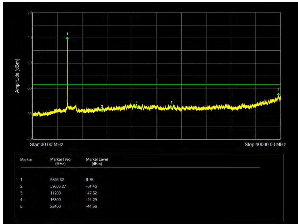
Tx. Spurious NVNT 802.11ac20 5700MHz Sum Emission
