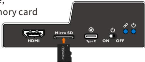
Please hold the edge of Micro SD card and please be aware of the label direction. Insert the card with the connector end toward the slot until the memory card is secured inside the slot.
