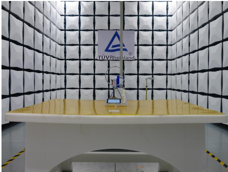
Photograph 1: Set-up for Radiated Spurious Emission, Below 30MHz
