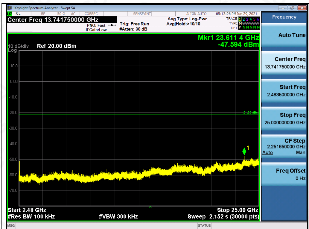
Test_Graph_LE1M_ANT1_2402_1Mbps_Higher Band Emissions
