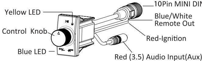
**WARNING** -When attaching RED ignition wire you will by-pass the internal On/Off switch
