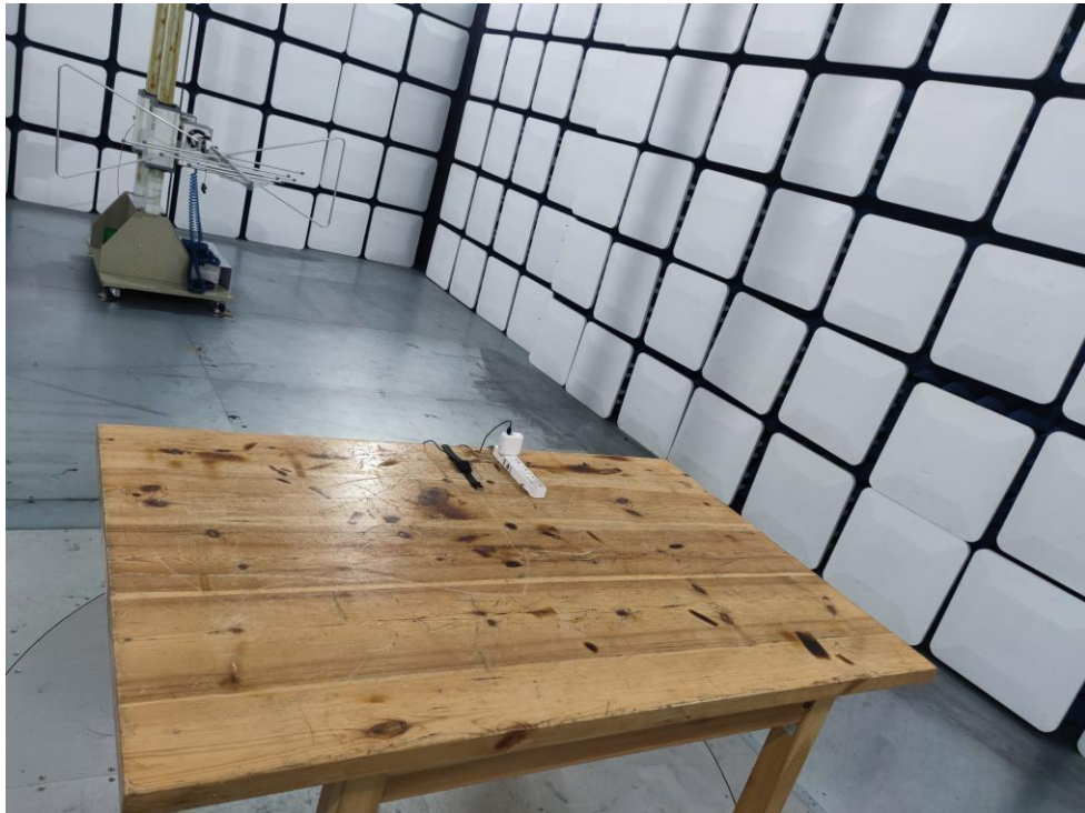
Photo of Radiation Emission Test
