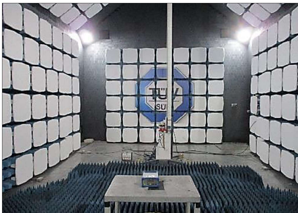
Figure 13 - Test Setup - 1 GHz to 13 GHz
