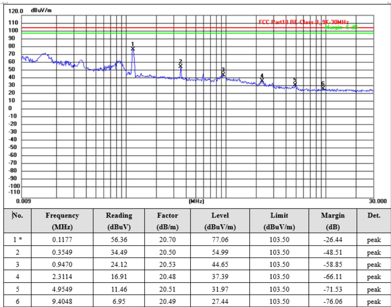
Remark: Measured at antenna position 0 degree and 90 degree, recorded worst case at 0 degree.
