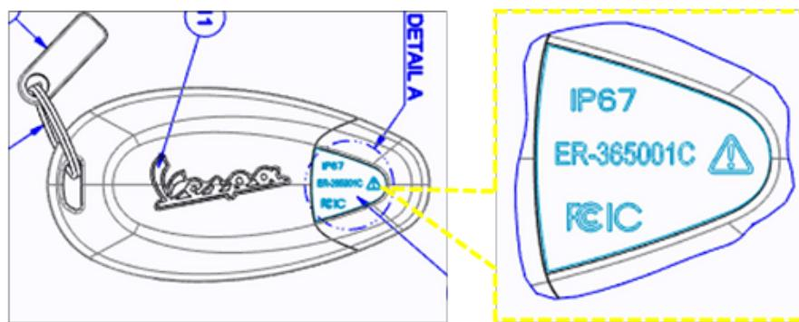
FCC and IC Certification no. will be on user manual as well as product shipment package due to limited space of the small size device
