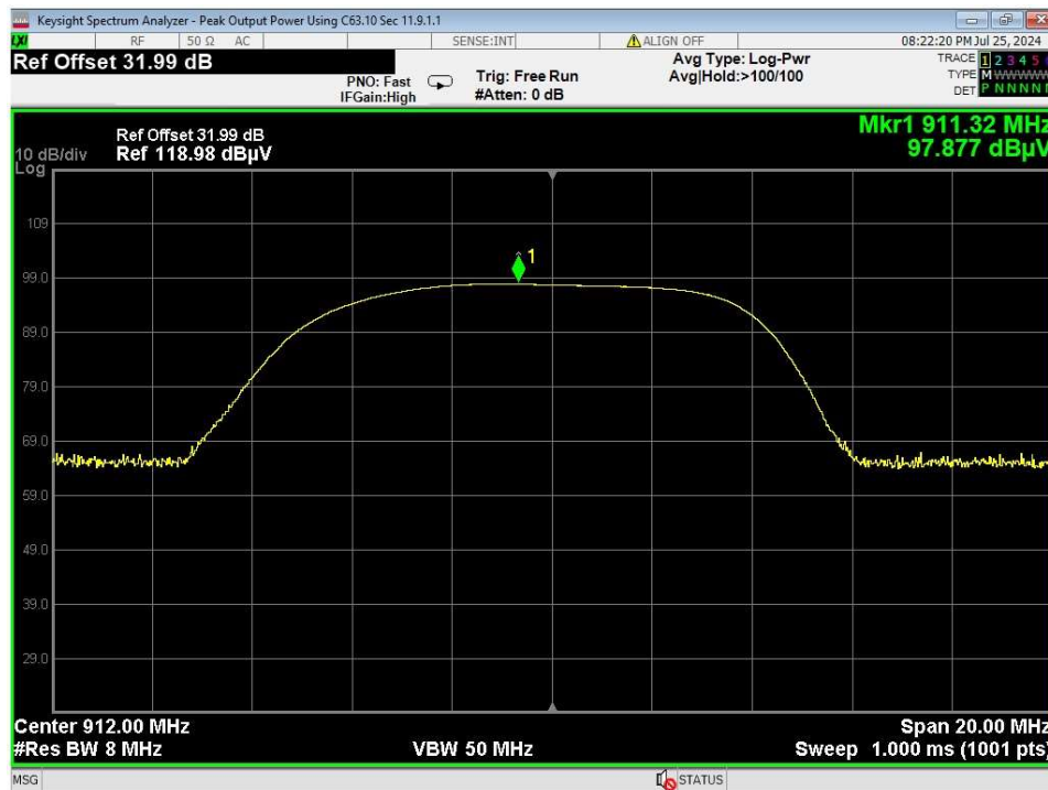
Figure 13 – Peak Field Strength, Low Channel.
