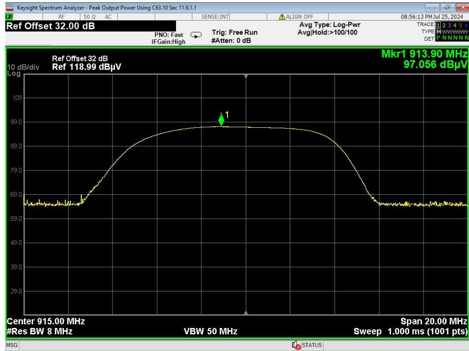
Figure 14 – Peak Field Strength, Mid Channel
