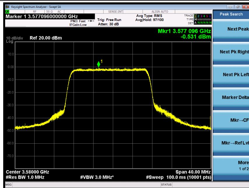
EIRP PSD=-0.563-0.63+4.5=3.307dBm/MHz, Antenna gain is -0.63dBi, the path loss is 4.5dB
