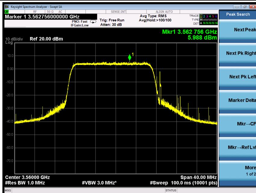
EIRP PSD=5.988-0.63+4.5=9.858dBm/MHz, Antenna gain is -0.63dBi, the path loss is 4.5dB
