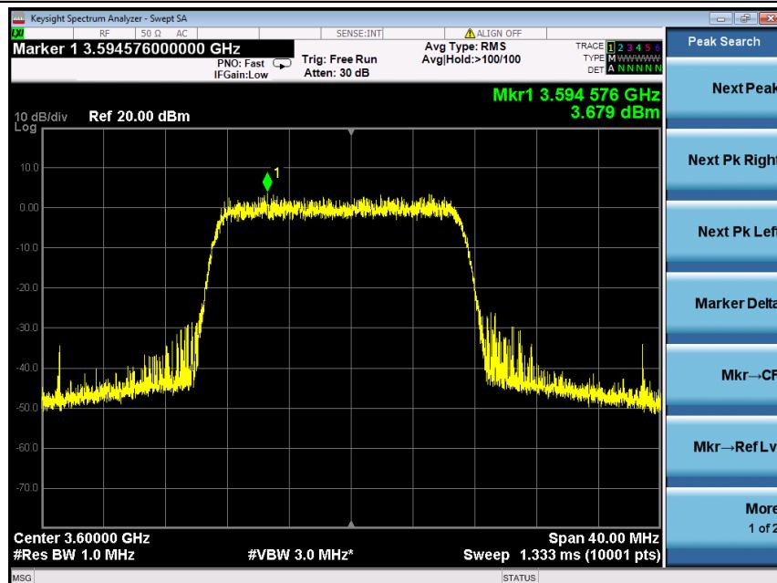
EIRP PSD=-3.679-0.63+4.5=7.549dBm/MHz, Antenna gain is -0.63dBi, the path loss is 4.5dB,
