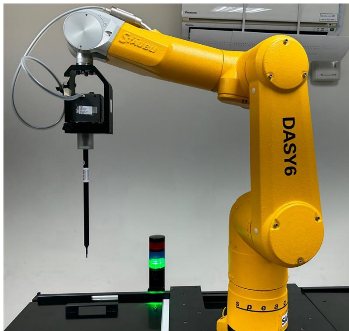
Fig.1 Photograph of the SAR measurement system
