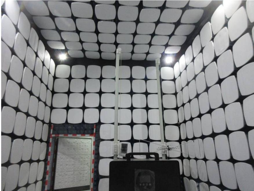
There is a holder to keep the height of the antenna of the EUT is 1.5m.
