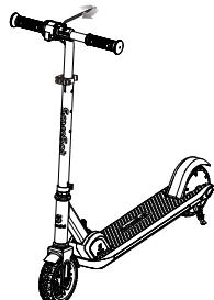
4. Using the 5mm Allen Wrench tighten the handlebar clamp.
