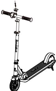
3. Insert the handlebar with the throttle facing the rider.
