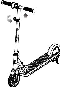
5. To adjust the height of the handlebar, open the quick-release lever and slide the T-bar to the desired position and resecure the quick-release lever to lock into place.
