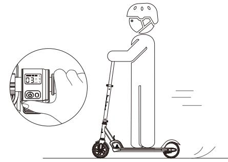
3. When the scooter starts to coast, put both feet on the deck and push down the accelerator.
