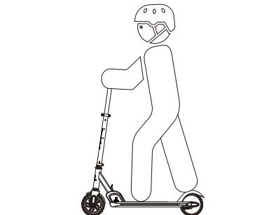
5. For controlled stops, release the throttle and apply the brake by putting pressure on the rear-fender brake.
