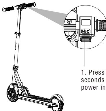
1. Press the power button and hold for 2 seconds to turn on the scooter. Check the power indicator.
