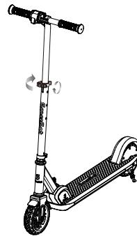
6. The tension of the quick-release lever can be adjusted by manually tightening or loosening the Allen bolt. Be careful not to overtighten. You should always be able to open and close the quick-release lever by hand and the T-bar should slide freely when the quick-release is open.
