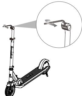
2. Using the 5 mm Allen Wrench loosen the handlebar clamp.
