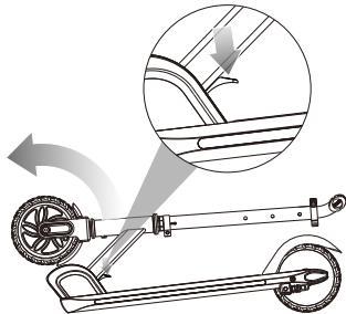
1. To release the folding mechanism, place the scooter on the ground, push the release lever down to unfold the scooter.
