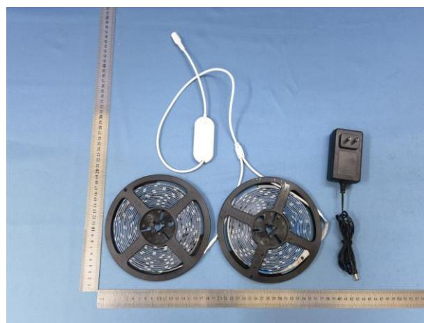
Model No. 900-00076\_A, QS-338SL-1 the only One light strip; the model of adapter is HP18A-1201500-AU; The rated power is 18W.
