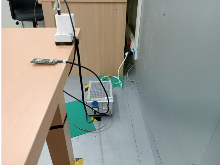
Photograph 5: Test Setup for Mains Conducted Emissions (Back View)
